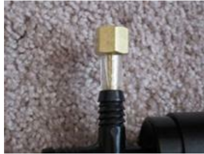
Figure 4. Wrap some tubing around the barb to get a snug fit and insulate the plastic from heat.
