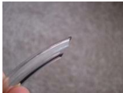
Figure 5. Cut the tubing at an angle—this will allow you to wedge it into the blower tube.
